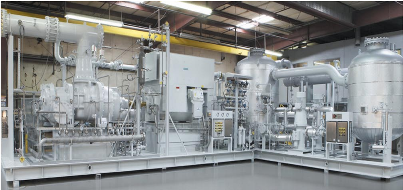
Figure 1. Typical oil injected screw compressor package for refinery PSA unit, hydrogen tail gas service.
