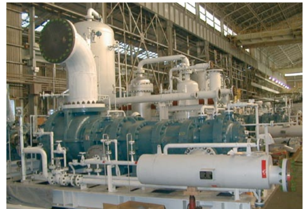
Figure 6. Hydrogen (99.5%) booster for dissociation process.
